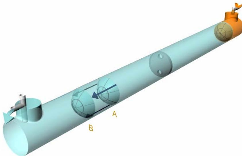
**Figure 2** - Closed-conduit flow tank during 10% volume dosing of 120 gallons with 'untreated
