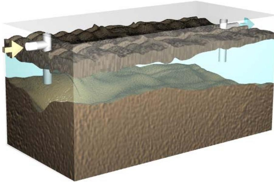
**Figure 4** - Conventional tank F3 with 64% solids after 6 months of 750 gpd dosing in Study 1. Note heavy scum formation at airspace.
