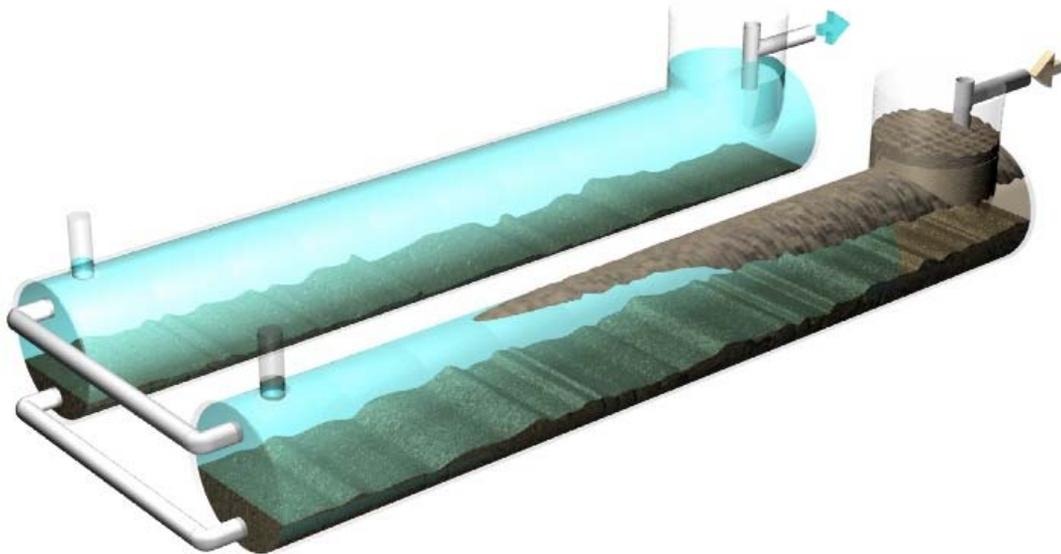
**Figure 5** - 'Flooded' tank A3 with 30% solids after 6 months operation in Study 1 (included 5 months of 750 gpd dosing and 1 month at 1500 gpd not included in analytical results) . Note lack of scum in flooded section of tank.
