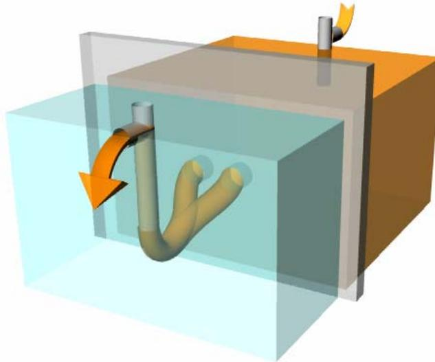
**Figure 1** - Conventional 1200 gallon Ontario CSA septic tank with 2:1 compartments and 6” central orifices in partition during 5% and 10% volume dosing (Lay et al., 2005), showing upwelling into airspace above the invert of the outlet pipe, and the resulting visible 'untreated sewage' plume formed directly from inlet, through partition orifices, to outlet.
