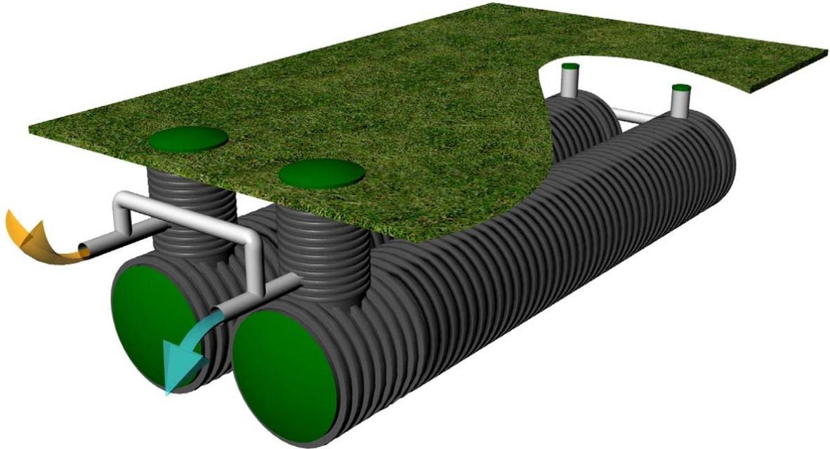
**Figure 3** - ‘Flooded’ or closed-conduit flow tank of 1500 gallons capacity tested side-by-side with 1500 gallon conventional single-compartment tank at Buzzards Bay test facility. Water level is 3 inches up into risers, controlled by the outlet invert (blue arrow). Submerged or flooded flow between the inlet (brown) and outlet risers acts to restrict hydraulic short-circuiting and form of scum.
