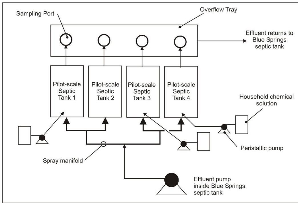
**Figure 2. Layout Schematic of the Experimental Apparatus**
