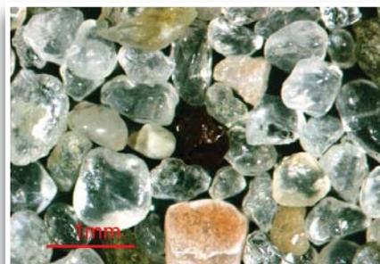
Figure 2. Clear sand is a standard medium used for filtration of sewage. Microbial biofilm coats the sand grains as wastewater moves down through the narrow interstices between grains. Only treated effluent enters the natural environment.
