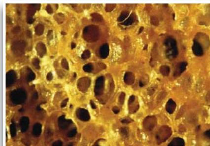
Figure 3. Beneficial microbes colonize interior surfaces of Waterloo Biofilter absorbent medium, and grow out into large open pores, allowing 10 times the loading rate of sand without plugging, with the same high-quality effluent.
